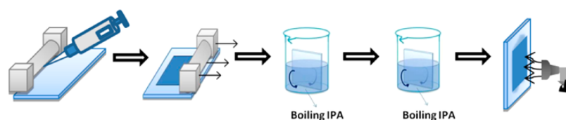
Figure 1. Processes involved in the blade-coating method. The PS suspension is blade-coated on the substrate, and then the substrate is dipped into a beaker of boiling isopropanol to remove the PS spheres in the bladed ethanol layer. The substrate is moved to another beaker of boiling isopropanol and blown dry after 10 s.
